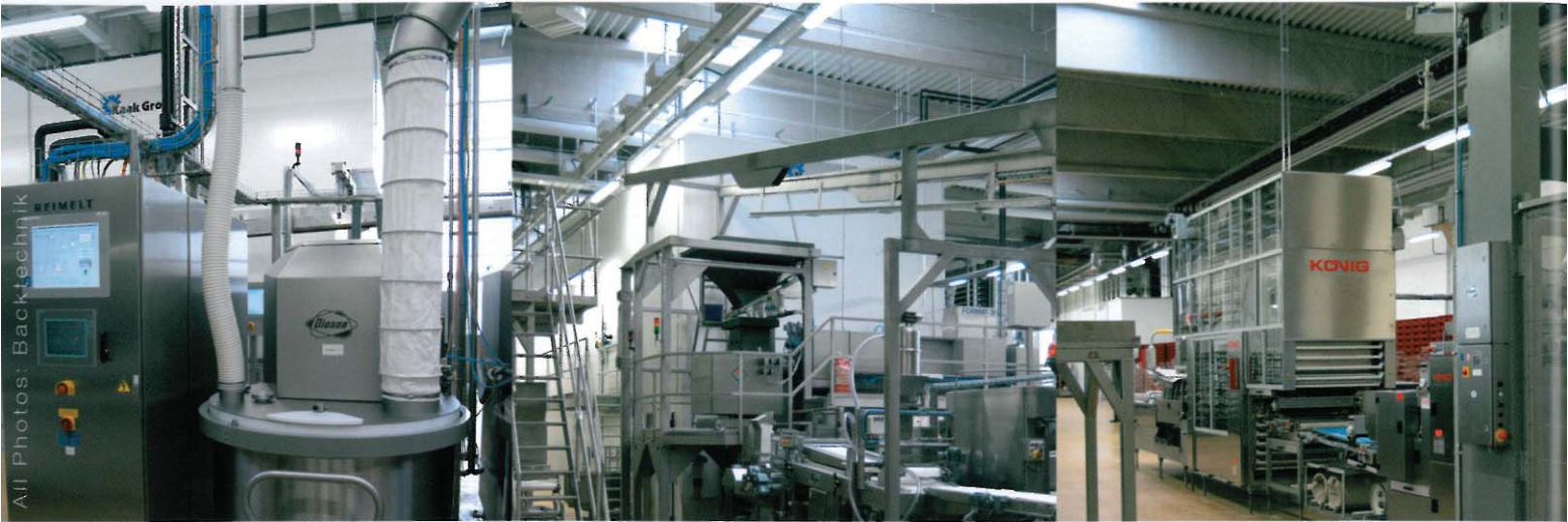
Left: Even in the kneading technique sector, the production is optimally equipped. Depending on the dough, spiral and wendel kneading machines by Diosna are installed. Middle: Bread and tin bread line by Kaak. Right: Almost all well-known suppliers delivered equipment to Bergkirchen. Here a bread roll line by König.
