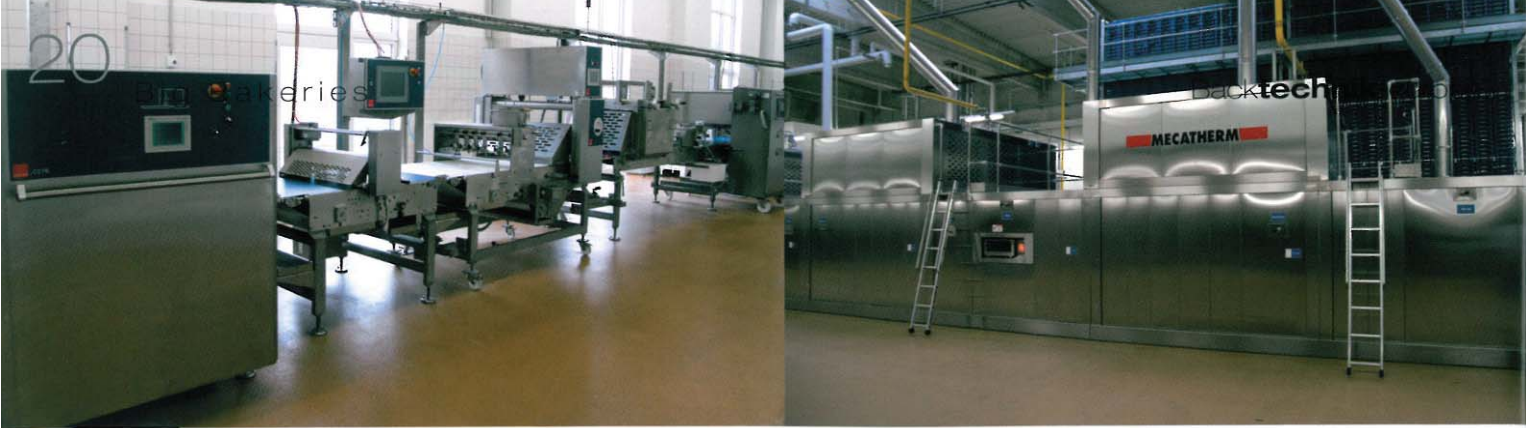
Left: In a separate, air-conditioned room, pastry products are produced on a Fritsch line. Right: The Mecatherm tunnel oven with the new paternoster-system in the background.
